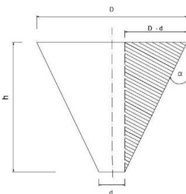
Figure 2: Basic dimensions of a truncated cone.
