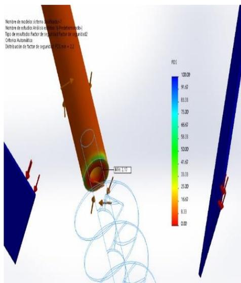
Figure 5: Safety factor in the dosing system
