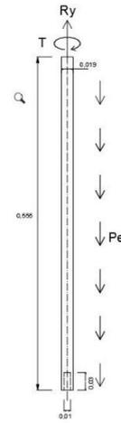
**Figure 4: Diagram free hub body**
