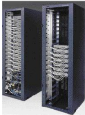
Figure 4.2 Stacking solution of AS 5300
