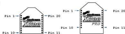
Figure 1-03. XBee/XBee-PRO RF Module Pin Numbers
