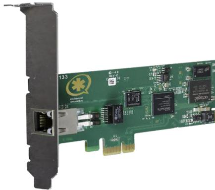
Figura 8: Tarjeta E1 Fuente: <https://www.digium.com/products/telephony-cards/digital/single-span>
