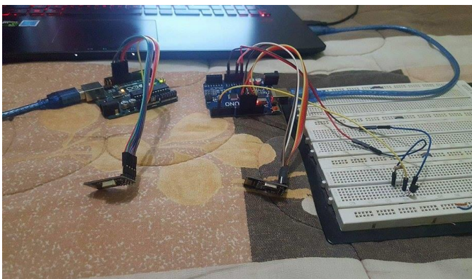
Figure12. Sensor network using RF modules. Source: Authorship.
