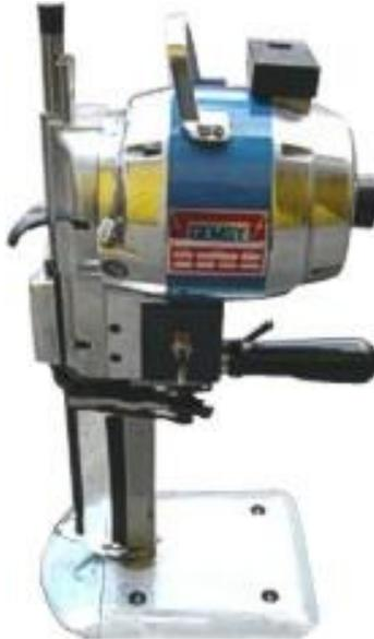
**FIGURA 22:** Máquina De Corte Vertical
