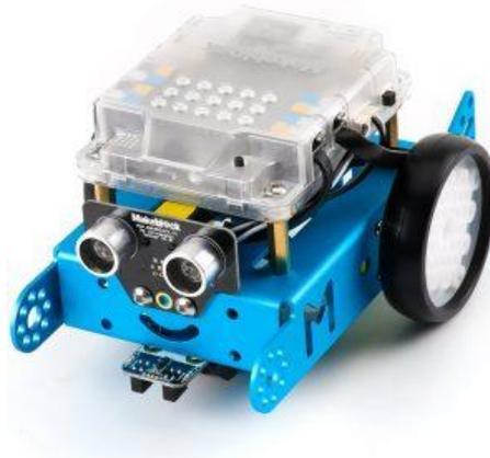
*Figura 11. Robot mBot de Makeblock*
