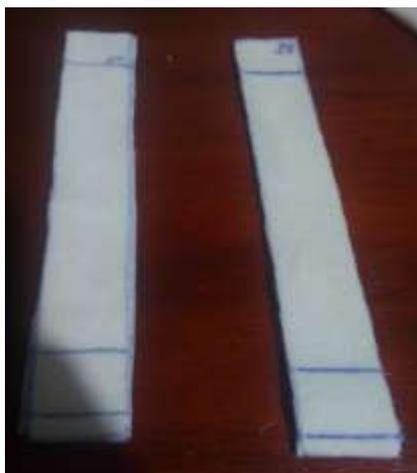
**Figura 39** *Probeta 100% Pes Pique*
