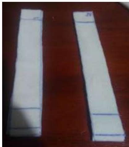
**Figura 35** Probeta Jersey Simple 100% CO
