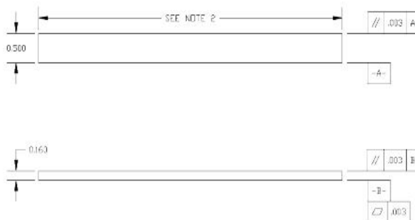
FIG. 5 Standard Flexural Test Specimen Drawing (Inch-Pound)
