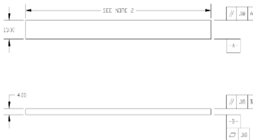
FIG. 4 Standard Flexural Test Specimen Drawing (SI)
