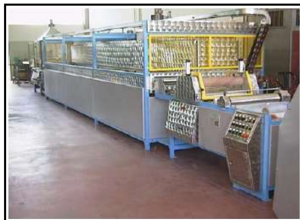
Figure: Bonding machine of three furnaces
