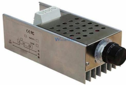
*Figura 11: High Power Dimmer AC 110V 220V 10V 10000W SRC [29].*
