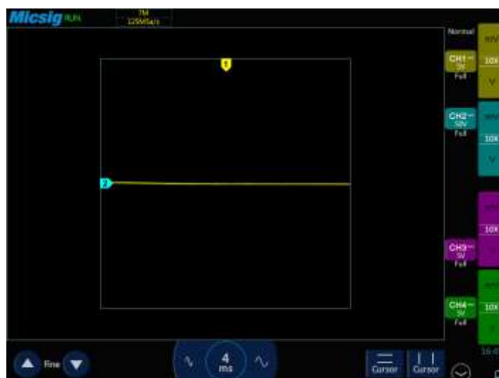
Figura 3.27 Oscilograma pines 1, 2, 3, 5, 9, 10, 11, 14 y 16 Socket B
