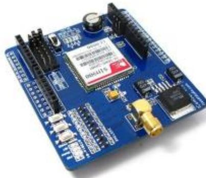
GPRS module is a GSM/GPRS module based on the SIM900 Quad-band GSM/GPRS module. It is controlled via AT commands (GSM 07.07 ,07.05 and SIMCOM enhanced AT Commands), and fully compatible with Arduino / Iteduino and Mega.
