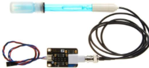
If pre-programmed, you will get the pH value easily. Comes in compact plastic box with foams for better mobile storage. **Attention: In order to ensure the accuracy of the pH probe, you need to use the standard solution to calibrate it regularly. Generally, the period is about half a year. If you measure the dirty aqueous solution, you need to increase the frequency of calibration.**
