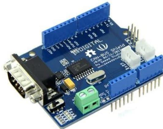
**Figura 2.5** CAN – Bus Shield V2 MCP2515
