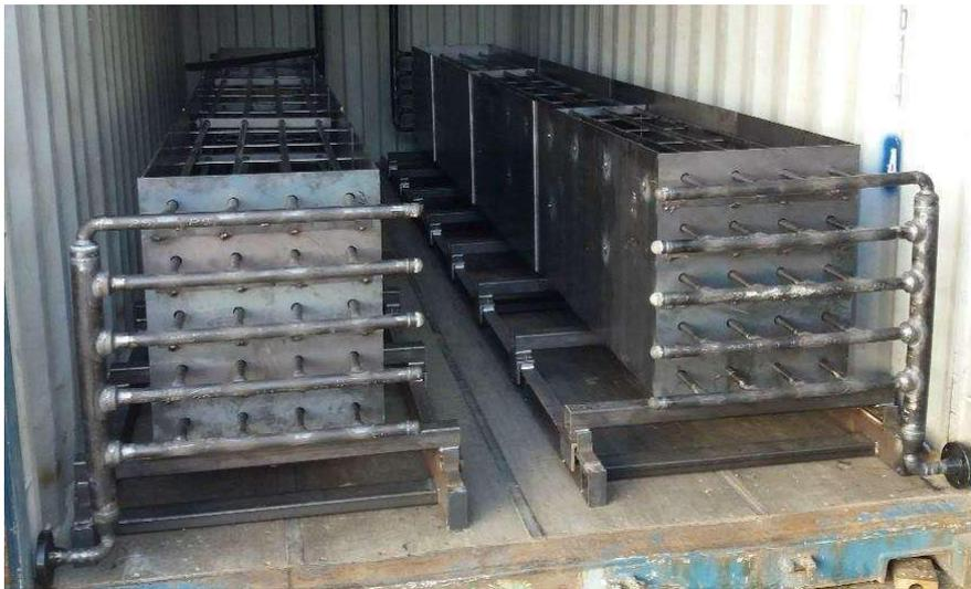
Fig. 3.1 Módulos de solidTES (62KWt - 300 KWh),
