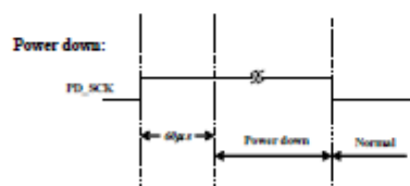
Fig.3 Power down control
