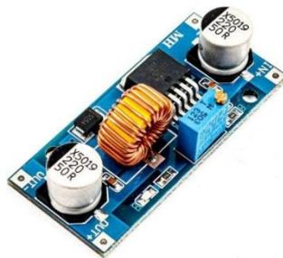
Fuente: (XLSEMI, 2017) Datasheet 5A 180KHz 36V Buck DC to DC Converter XL4015. [www.xlsemi.com](http://www.xlsemi.com)
