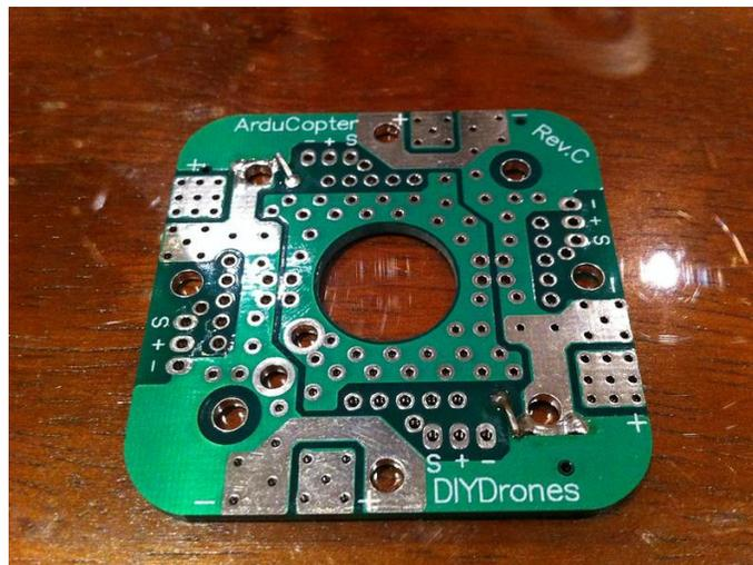
Figura. 16 Power distribution board. Fuente: (Kvisberg, 2011).
