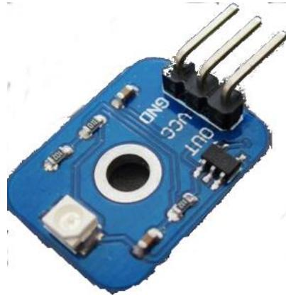
Adaptado de *Sensor GUVAS12SD* por Kakao Corp, 2020, Arduino Sensor for Everyone (<https://arduino.steamedu123.com/entry/GUVA-S12SD-Ultraviolet-Light-Sensor>)
