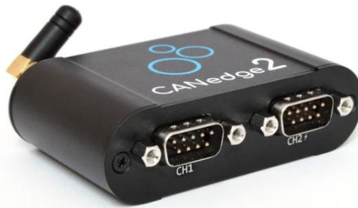
Figura 2.3 Datalogger CANedge2 (CSS Electronics, 2022)
