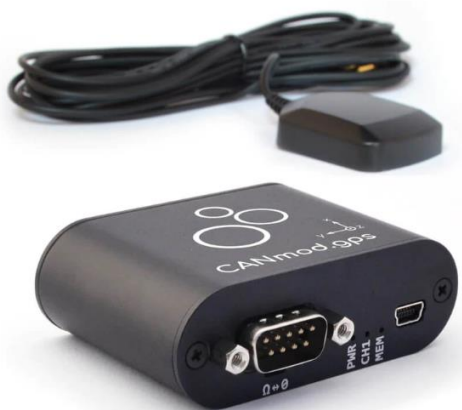
Figura 3.4 GPS a CAN con sensor inercial 3D y UDR (CSS Electronics, CANmod GPS-to-CAN , 2022, pág. 6)
