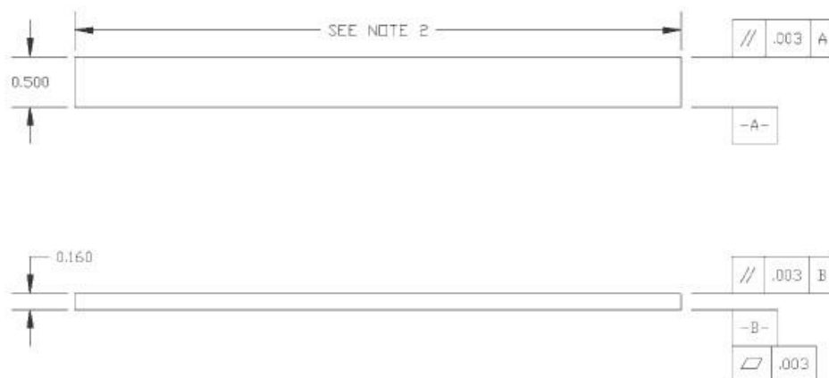
FIG. 5 Standard Flexural Test Specimen Drawing (Inch-Pound)
