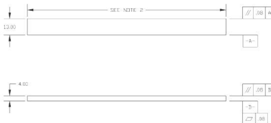
FIG. 4 Standard Flexural Test Specimen Drawing (SI)
