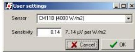
Use the wizard to select the sensor model that is to be used, and then enter the sensitivity of the sensor. The LI-19 is then ready to be programmed with the new settings. To do that, click the 'Program' button.
