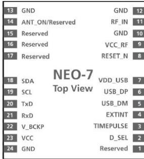
Figure 2: Pin Assignment
