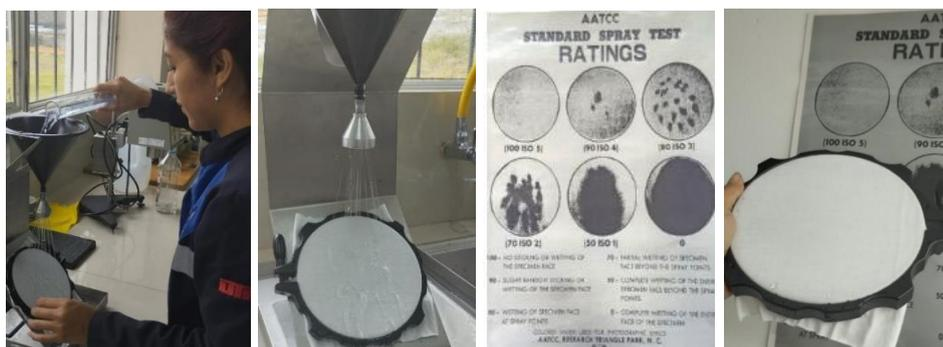
**Figura 15***Prueba de lavado doméstico ISO 6330*
