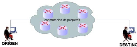
Figure 3. Packet switching network between users.
