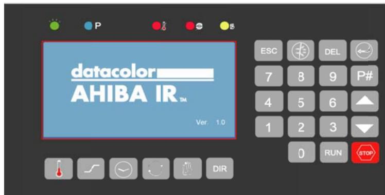
Fig. 29 Controlador Principal del AHIBA IR
