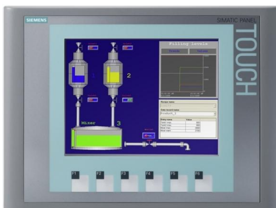
Figura 5.1. HMI Simatic KTP600
