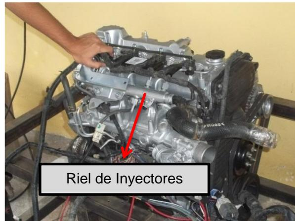
Figura. 65 Motor Common Rail
