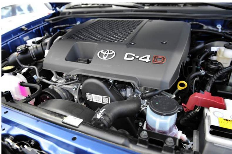
Figura. 4 Motor Toyota Hilux Diesel 2.5 D-4D GX
