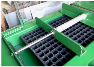
Figure 4. Pneumatic cylinder for the opening and closing of the mouth of the hoppers
