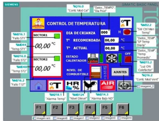
Figure 24.-Temperature Control System Screen
