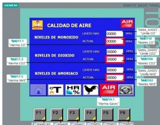
Figure 27.-Gas Monitoring System Screen
