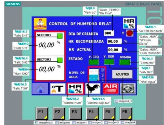
Figure 25. - Humidity Control System Screen
