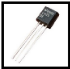
Figure 14. LM35 temperature sensor. Source: LM35. Retrieved from: http://www.rapidalph.com/shop/lm35-temperature-sensor/
