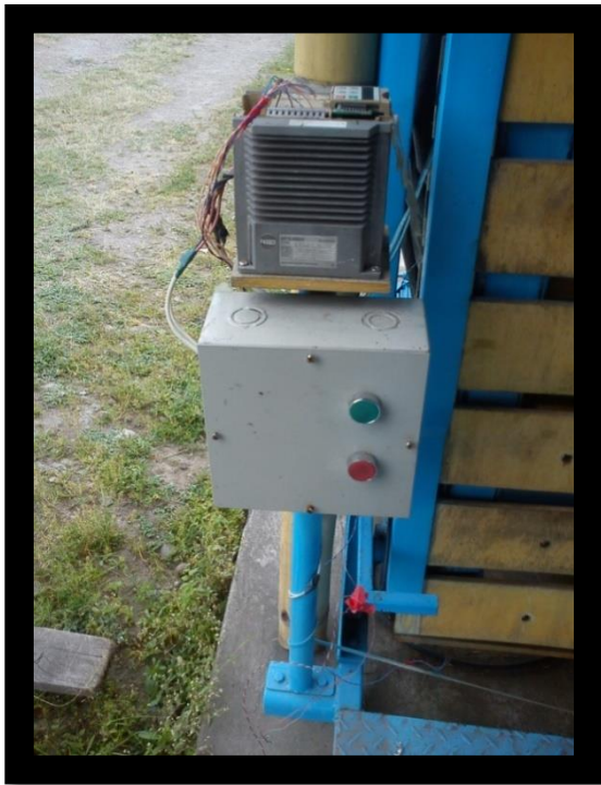
Figure 4.1 Mounting the drive and speed buttons on and off
