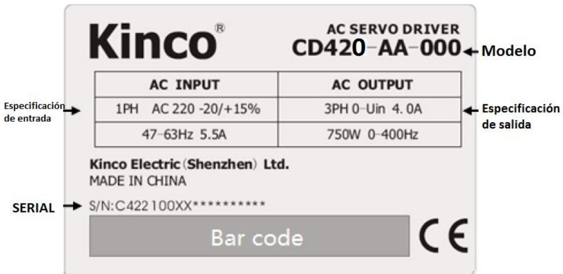
Figura 71. Placa del servomotor, Kinco Automation
