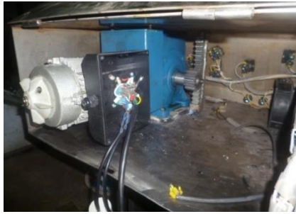
Figure 18 Mounting the gear motor, rack and pinion
