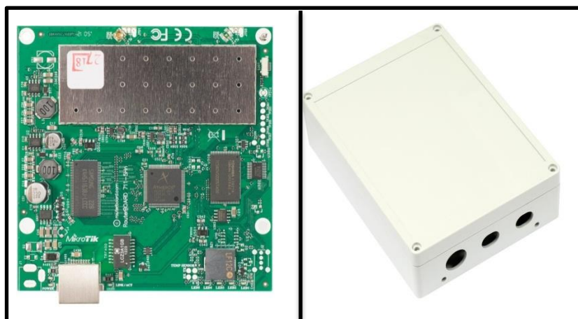
Figura A 5. RouterBoard – RB711-5HnD
