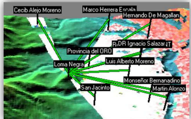
Figure 19: Coverage area of the 120° sector antenna and directive antenna Node Loma Negra; Radio Mobile software simulation.
