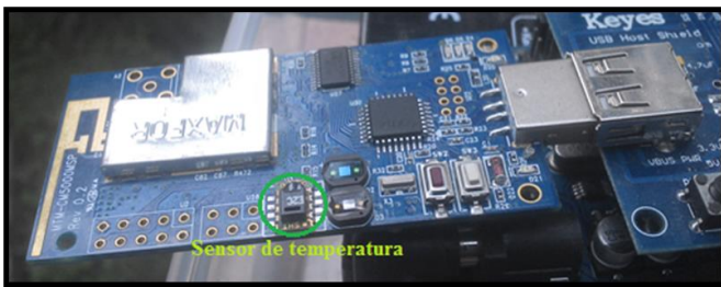
Fig.29 Identification of the temperature sensor installed in the sensor node
