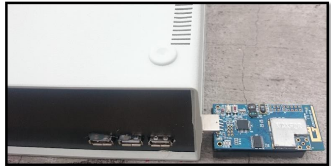
Fig.33 Server node connected to the gateway
