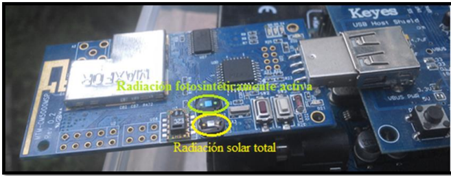
Fig.30 Identification of solar radiation sensors installed on a sensor node
