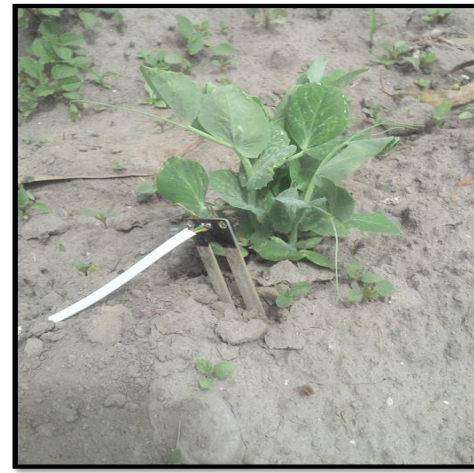
Fig.32 External soil humidity sensor in a sensor node installed
