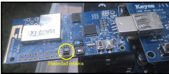
Fig.31 Relative humidity identification sensor in a sensor node installed
