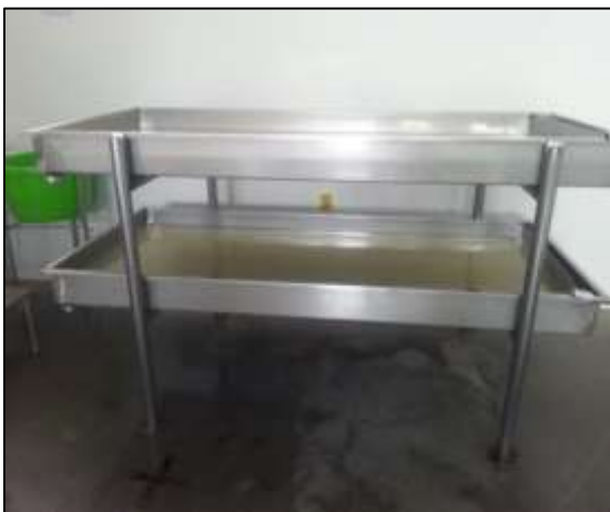
Figure. 6. Salero of stainless steel material Source: Company "Dairy Products Yaznan". Developed by: Mariela Cepeda
