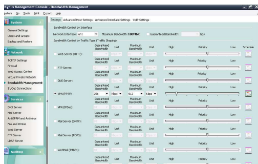
Figure 6. Allocation of bandwidth for VPN Reference: KYPUS captured image server
