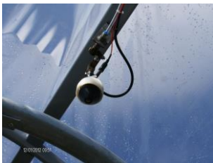
Figure 7. Electrostatic spraying nozzle
