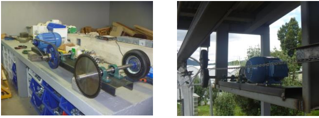
Figure. 4. Traction system, drag chain drive
