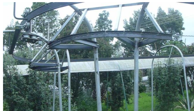
Figure 3. Transport system for cars with flowers cut into the tunnel of fumigation
