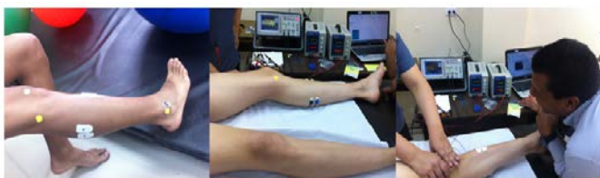
Fig. 22. Preliminary tests of SEMG system.
