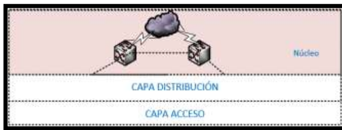
Figure 5. Layer Core the hierarchical network model Source: http://goo.gl/4clyx0 Modified by Esmeralda Patiño
