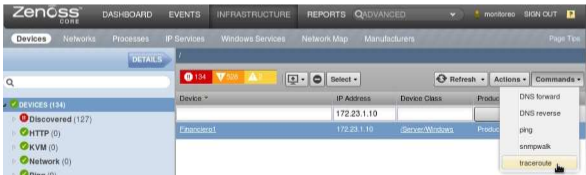
Figura 82. Ventana Commands Traceroute.
