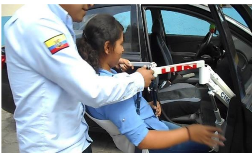
Figure 11. Person 2 with harness hooked to the transfer device
