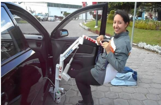
Figure 12. Person 3 with harness hooked to the transfer device.
