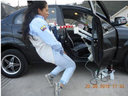
Figure 10. Person 1 with harness hooked to the transfer device.
