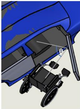
Figure 1. Angle between the center of the chair seat and the center of the vehicle seat.
