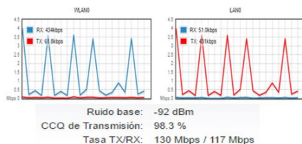
Figura 9. Throughput Station, Enlace Edificio Central UTN – COLEGIO UNIVERSITARIO Source: Technica University North
