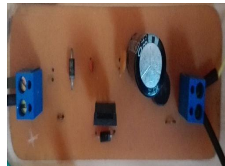
Figure 8. 9v fixed voltage source for the Arduino module
