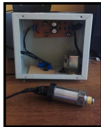
Figure 13. Industrial panel # 3 current-to-voltage transformation system
