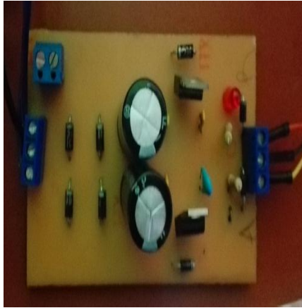
Figure 9. + -15 v voltage source for the pressure sensor
