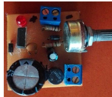
Figure 7. Variable voltage supply for SIM900 module Transmission and reception
