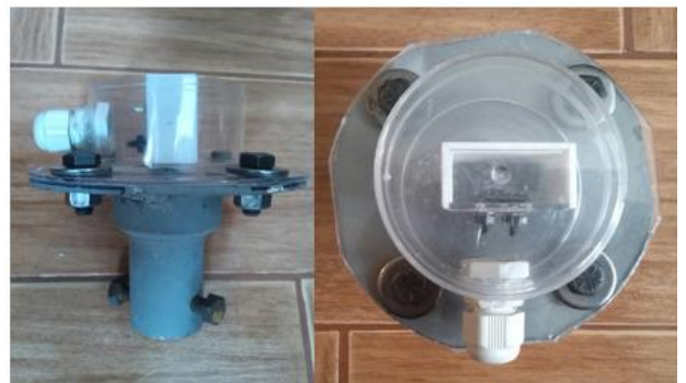
Fig. 7. Coupling and protective housing for the accelerometer.
