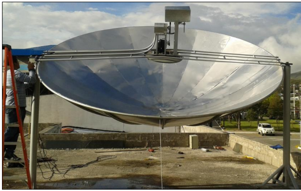
Fig. 3. Solar thermal generator of parabolic disk and stirling motor.
