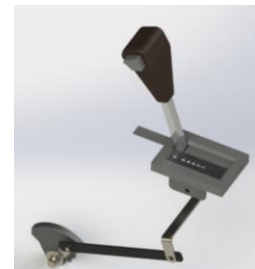
Figure 2. Adaptation of the selector lever.
