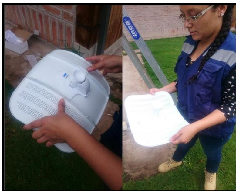
*Figura 58. Antena Litebeam M5-23 armada, Bosque Protector.*
